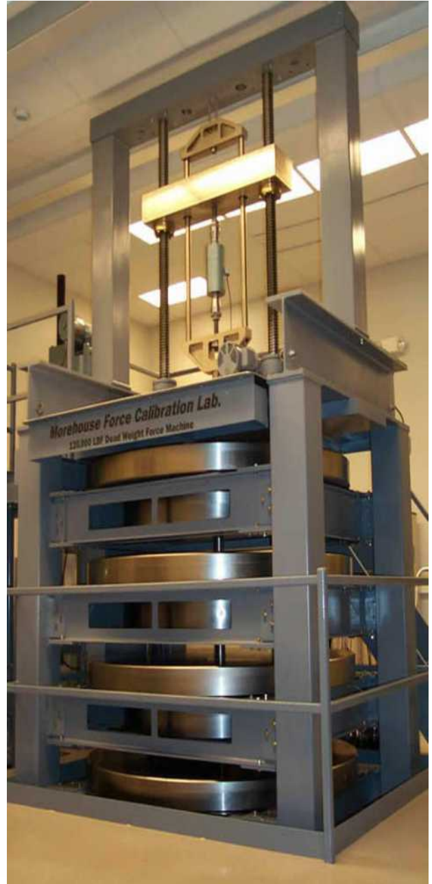
Morehouse Dead Weight Calibrator 1,20,000 lbf with CMC 0.0016% (Primary Force Calibration Reference Standard Installed at Morehouse Laboratory)
