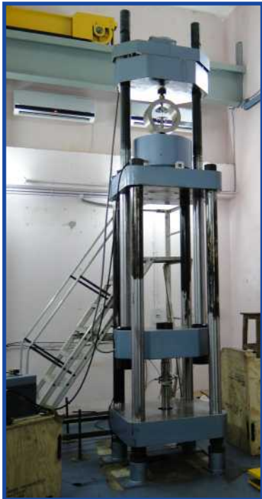
450 Ton Morehouse Load Cell Calibration Facility (having 0.025% uncertainty) installed & commissioned by Vaiseshika at Solid Motor Performance and Environmental Test facility, SHAR Centre, Sriharikota.
